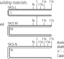
Available Crown Widths 1/4", 3/8", 7/16". 1/8" - 11/2" Lengths. Capacity 145-158.
